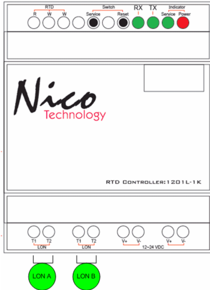
Figure 3.1 Connector pin assignment LonWorks network
